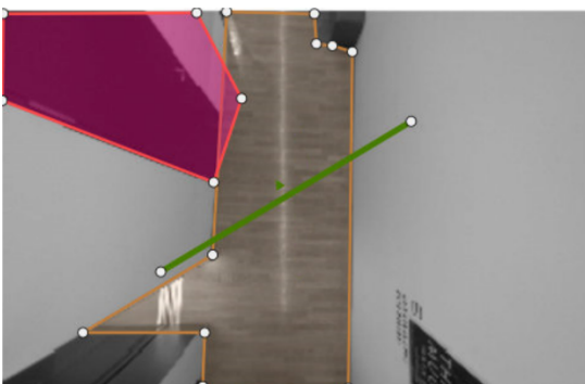
Figure 4-456: Final configuration with one counting line and masked door
